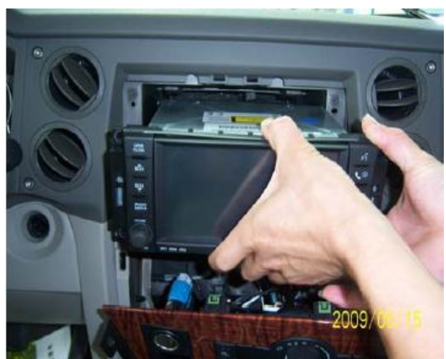
Loosen screws and pull out Monitor Deck (Comand)
