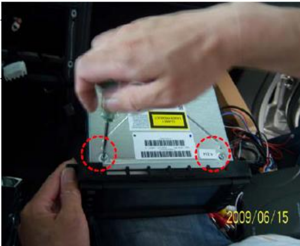
Loosen screws with case and separate LCD connector for install sub-board
